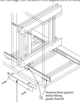
IMPORTANT: The guide channel height must be carefully adjusted to allow unrestricted forward movement of the Optimiser and to ensure the limit stop is held by the nylon wheel.
