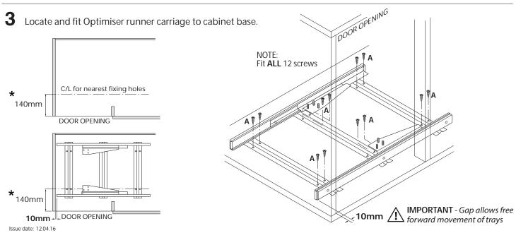
★ Doesn't apply to cabinets less than 500mm deep or cabinets without centre post.
