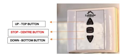
1. Press the downward direction arrow key once, to move the Loftrobe in downward direction from position **a**) **closed** to position **b**) **open** which stops as the motor reaches its pre-set lower limit. If you need to 'STOP' the unit from moving in a downward direction, press the 'STOP' button immediately (centre button).
